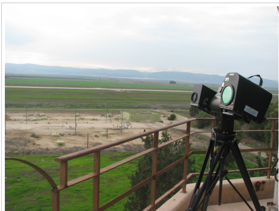
As well as identifying wildlife, Interceptor can also be used to detect any foreign objects on a runway and monitor aircraft traffic
