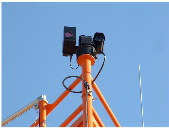
The Interceptor sensor unit mounted on top of an airfield antenna
