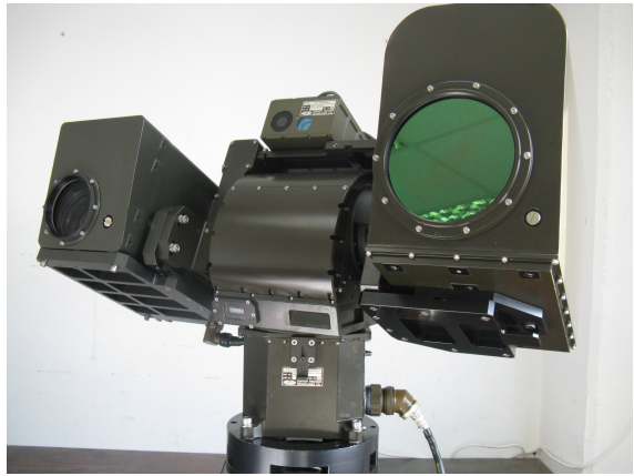
Interceptor's IR camera is located on the right side with a high powered CCD camera on the left. The long-range laser range finder is located on the top
